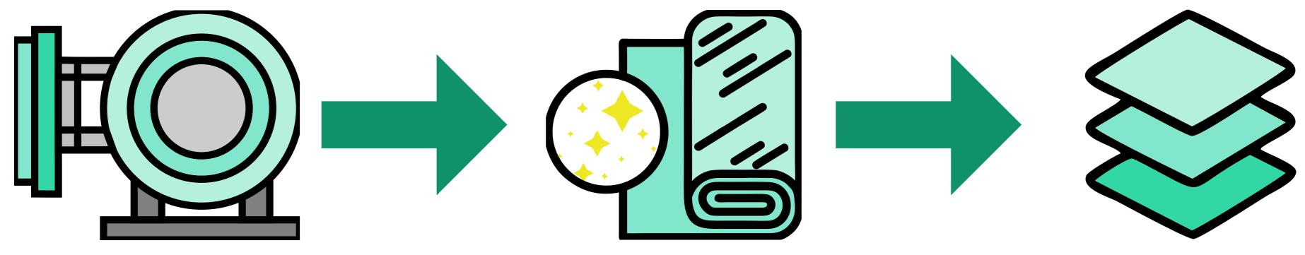
Supercritical Drying of an cellulose nonwoven precursor to solidify the nanoporous structure in the material
