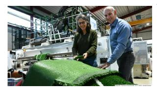
The aim of this development is an innovative, 100% recyclable artificial turf made from a group of materials (polyolefins). The material used for the polyethylene pile yarns comes from rapeseed oil and agricultural waste that does not compete with food production. The backing that holds the pile yarn in place is made of polypropylene (PP) and is stabilized on the reverse side by a recycled film made
