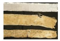
The evironmental challange of geotextiles is their "durability" as they are designed to last around 100 years. This meets the requirements for permanent structures, such as seawalls. However, for temporary applications, typically lasting one to two years, this durability is excessive and extends beyond the auxiliary function of the textile. In these cases, the materials remain in the soil without serving any further
